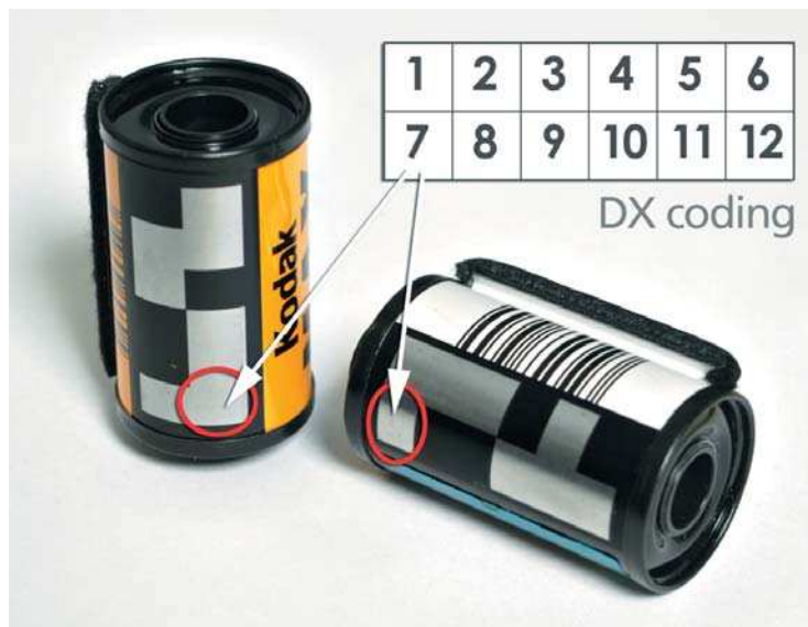
Figure 10.4 The DX coding on the outside of film canisters informs the camera about the characteristics of the film. The characteristics conveyed by each conductive position are: positions 1 and 7 always set; positions 2–6 used for ISO value; 8–10 for number of exposures per film; 11 and 12 for exposure latitude of the film.
